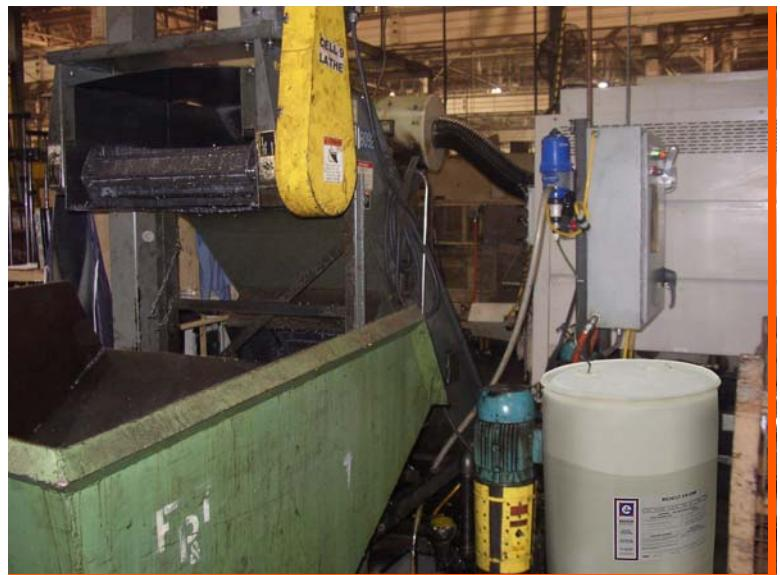
Consistent coolant sump levels are critical to maintaining proper chip flush and conveyor operation.
